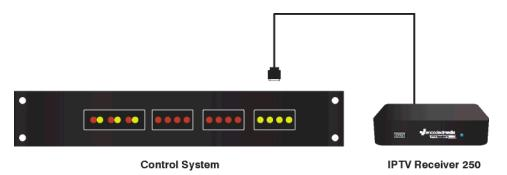
The RS-232 port is connected to the room control such as a Crestron® or AMX®.
