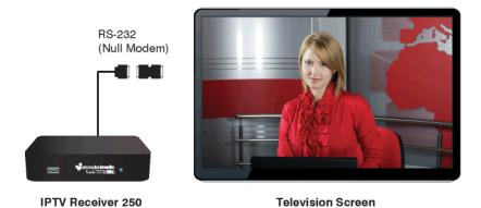
The RS-232 port is connected directly to the screen via the RS-232 port on the LCD, Plasma or Projector. In this configuration, the Receiver acts as an IP to RS-232 converter, allowing other authorised network devices to control and query the screen via an IP port.
